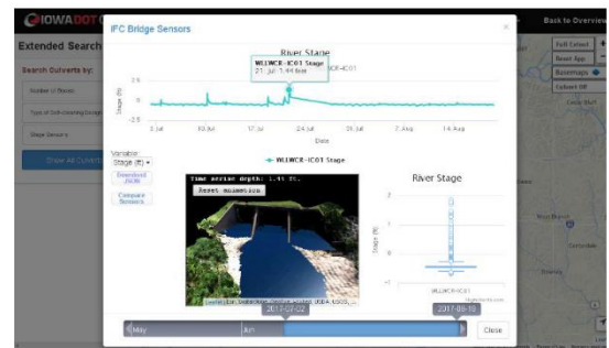
Time series of stage measurements visualized in a realistic digital culvert view
